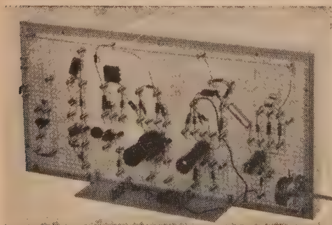
Vector Electronics 25X circuit mock-up board. Note the quick-clip solderless connectors.
