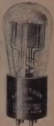
UV-200 detector tube. Similar in size to the 201As, these tubes were 50% more sensitive than crystal detectors.
