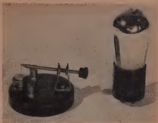
Comparison of a UV-201A receiver amplifying tube with a crystal detector.
