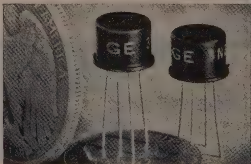
General Electric's new tetrode transistors are designed for use in rf, if osc. and mixer circuits.
