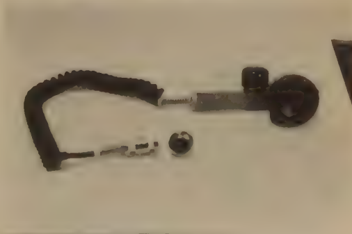
5—Microphone is reassembled and desired plug attached. Most T-17 microphones contain wire connection diagrams pasted inside of button switch.
