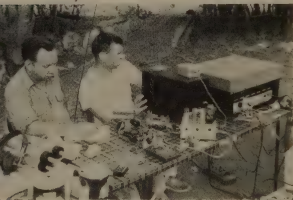
Jake operates while Frank keeps the log at the other station installed under a tree. Equipment is Drake receiver and HT-32. Antennas were dipoles hung from a 40 foot Tele-Vue crankup tower.
