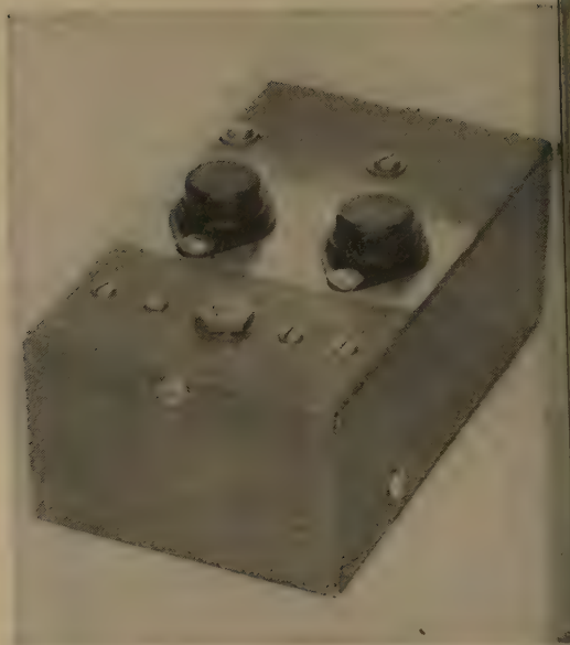
The transistorized 300 volt, 100 ma. power supply that was described last month. Somehow the photographs forgot to get in the envelope along with the manuscript.
