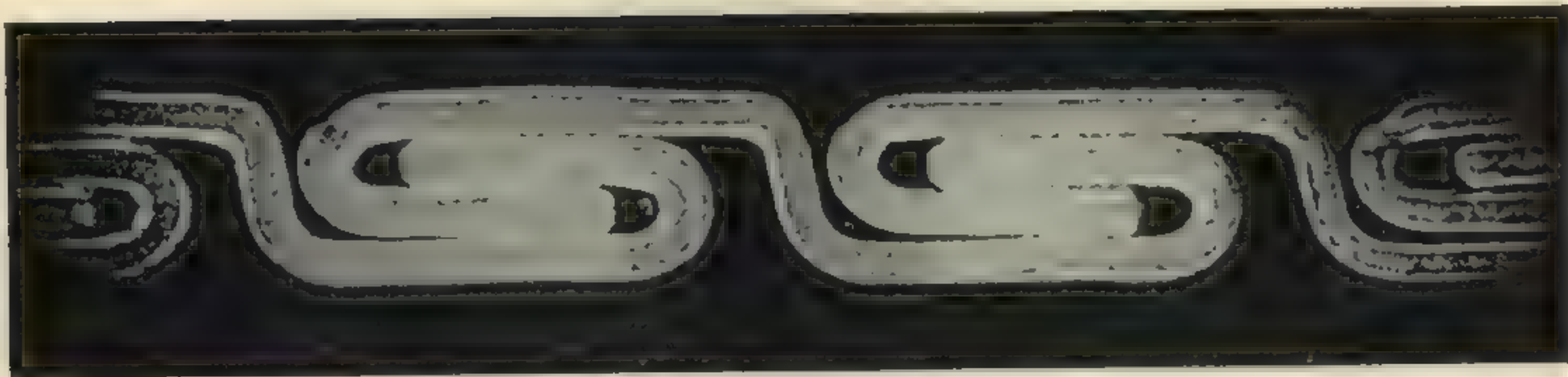
Fig. 1. Enlarged cross-section of silver-laminated-bronze interlock type of construction.
