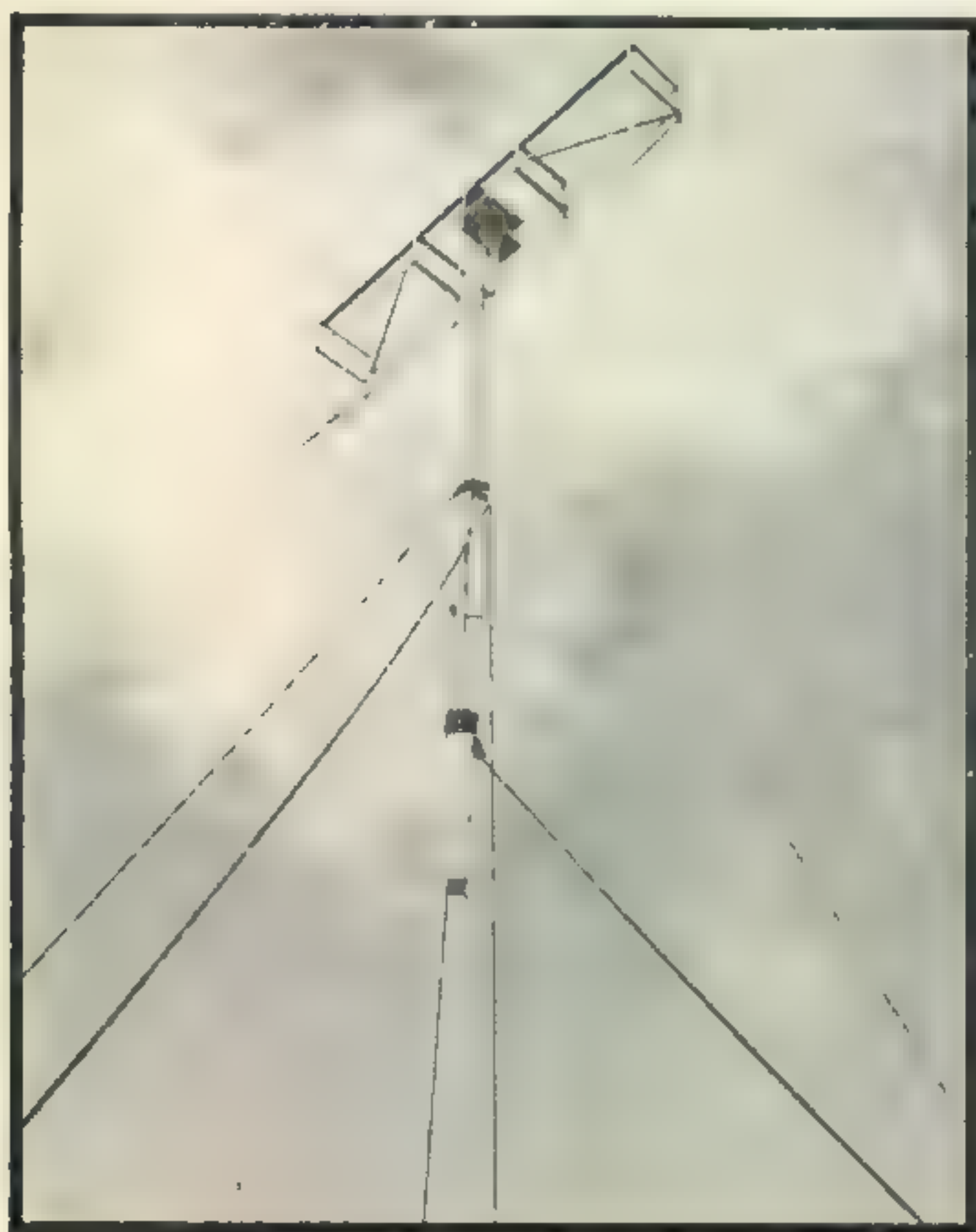
Eight-element antenna with "bed-spring" reflector on two meters at W3GKR.
