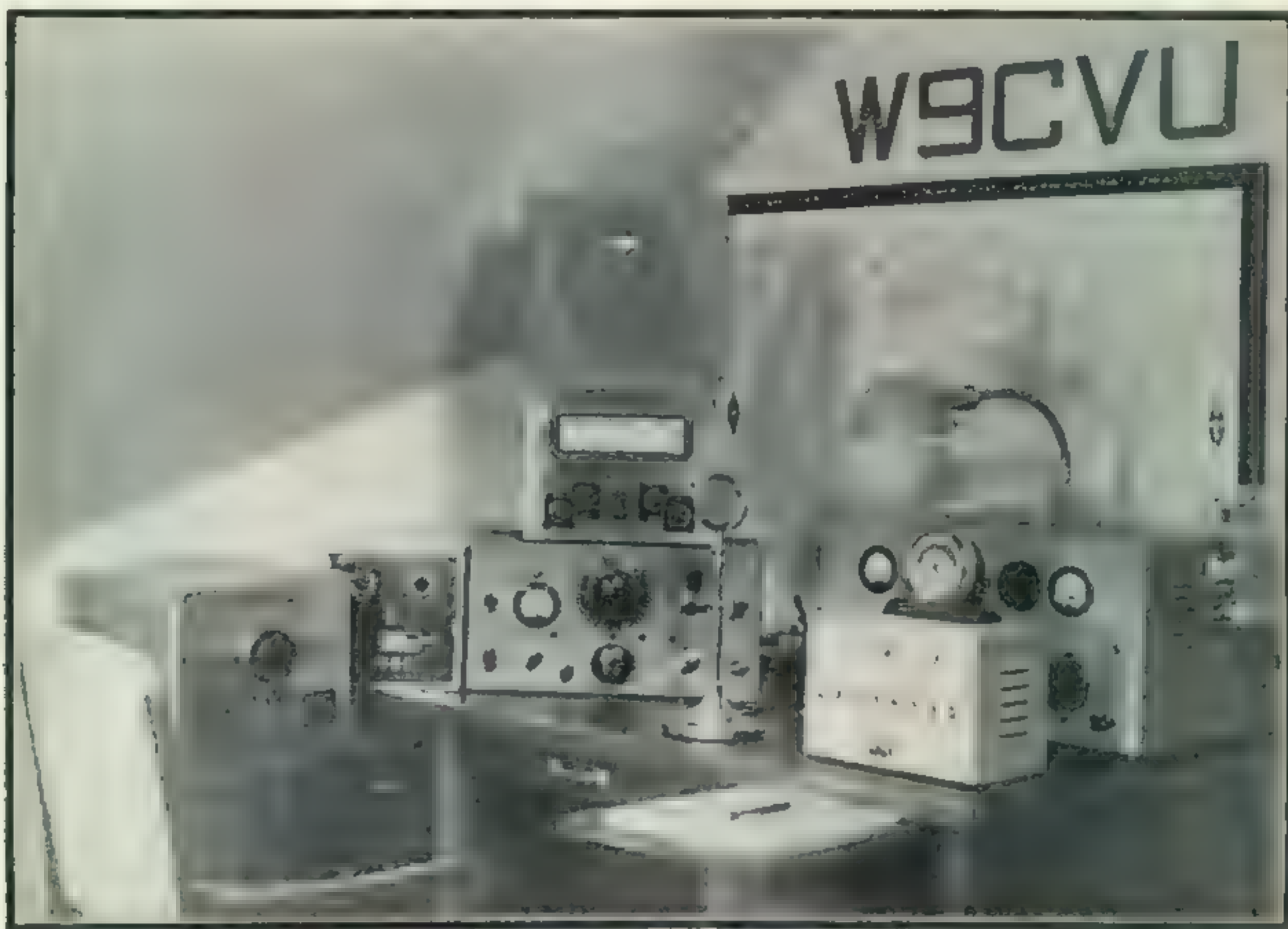
W9CVU puts a lot of equipment on a standard office size desk. The secret to this trick is absence of haywire of any sort. The practice of running control leads, interconnecting cables, etc. draped all over the shack should be number one taboo on the list of post-war station rules.
